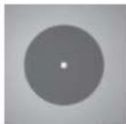
Figure 3 — Visual inspection of optical connector after cleaning with debris removed and improved metrics
