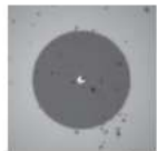
Figure 1 — Visual inspection of optical connector before cleaning, showing debris and poor metrics
